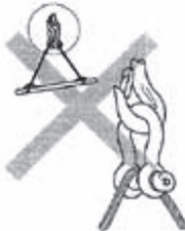
Figure 8: Wrong shackle rigging
