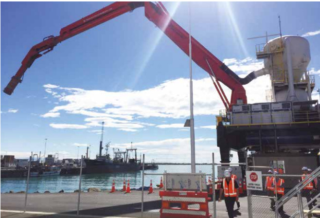
BULK MATERIAL AND LIVE STOCKS MANIPULATOR Working radius up to 44m.
