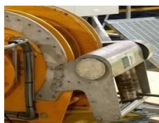
Spooling device (available as geared and auto-air)
